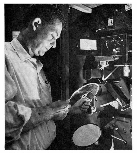
CLIFF FISK (9424) shows auxiliary computer equipment (part of the SC 4020) that exposes color film to make visual aids. Round cathode tube (bottom) produces image which is photographed through color wheel (in Cliff's hands) by camera mechanism at center top of cabinet. Cliff created general computer program which enables anyone to use the computer to produce drawings for slide resentations.
